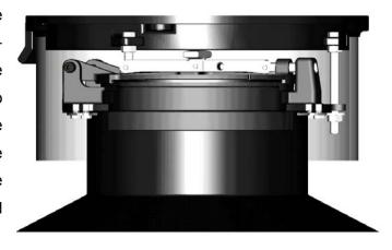
The Below Grade manhole also features an all-new rain tight bolt-cam action design with a hinged lid. It is interchangeable with all current bellow and bucket spill
