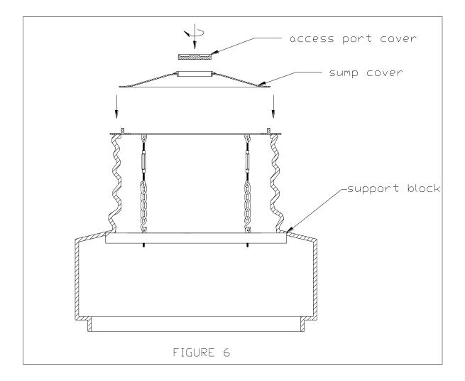
7. Secure the Sump Cover onto the Support Ring by screwing down with all 12 Wing nuts.
