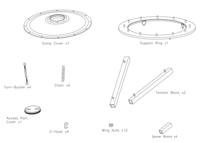
1. Determine if the Retrofit Cover will fit by measuring the diameter of the sump. Universal's Retrofit cover will fit sumps of diameter 27" to 34" as shown in Figure 1.
