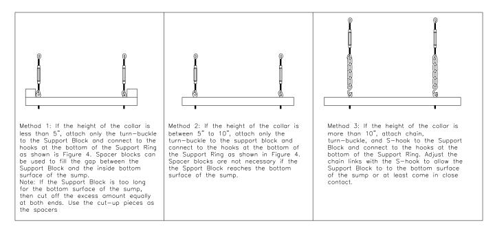
4. Make sure the hooks of the turn-buckle are fully extended by screwing outwards. Hold the chain assembly, and place it inside the sump and connect to the hooks of the Support Ring as shown in Figure 4 below.
