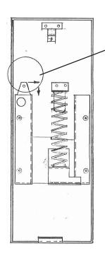
To Reset Cover: Insert a ball point pen point into the hole in the arm, move arm to the right and down. Cover is now reset and ready to use.
