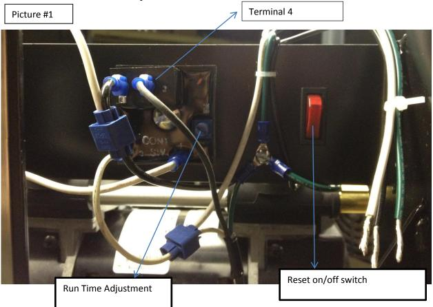
To make sure that the timer is working properly push the pushbutton switch at the front of the unit. There should now be voltage on terminal 4 in picture 1. If there is no voltage in terminal 4 then the timer needs to be replaced. The part number for the timer is 1975-15-A.
