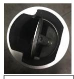
When testing the overfill valve the fuel level in the tank should be below the float (fully open valve) to ensure the full range of the float travel. The poppet should be in the position as shown in Fig.
