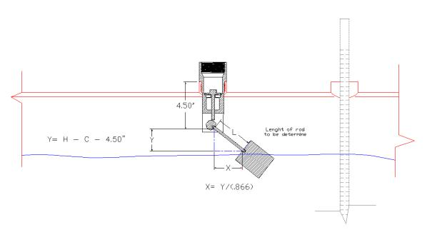
Figure 4 Calculating values for "Y" and "X"
