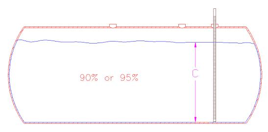
Figure 3 Height C for fill Capacity
