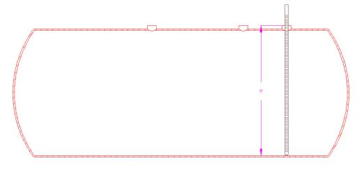
Figure 2 Tank Height Dimension
