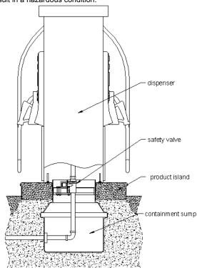
The shear section of the safety valve must be at the same level or no more than 1/2" above or below top of the dispenser base
