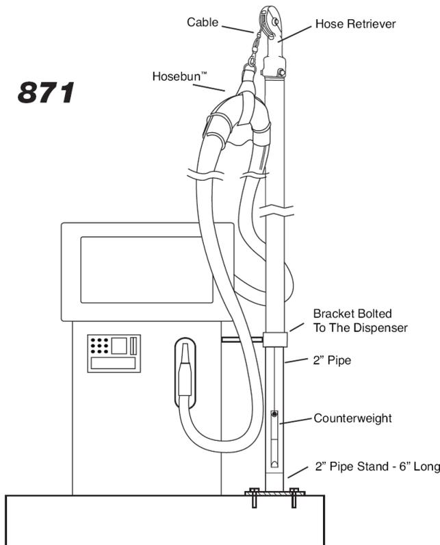
1. Obtain desired length of 2" schedule 80 steel pipe at any plumbing supply house.
