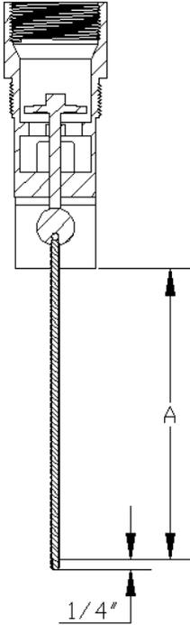
Figure 5 Length of Rod to be Cut
